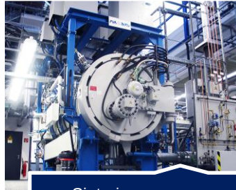
Sintering process up to 1,800 °C & 100 bar
