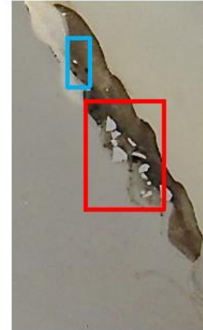
Figure 20: Macroscopic image of the Hardfacing, hard material particles (red), Hardfacing matrix (blue)
