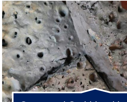
Cemented Carbide with broken bonds („Cake“)
